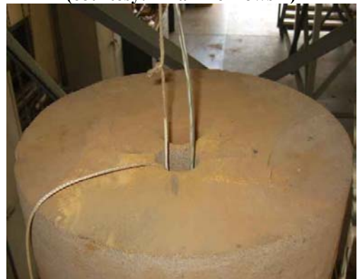
Figure 4: Top of borehole with umbilicals trailing down to fully submerged drill. (courtesy: Brian Derkowski)
